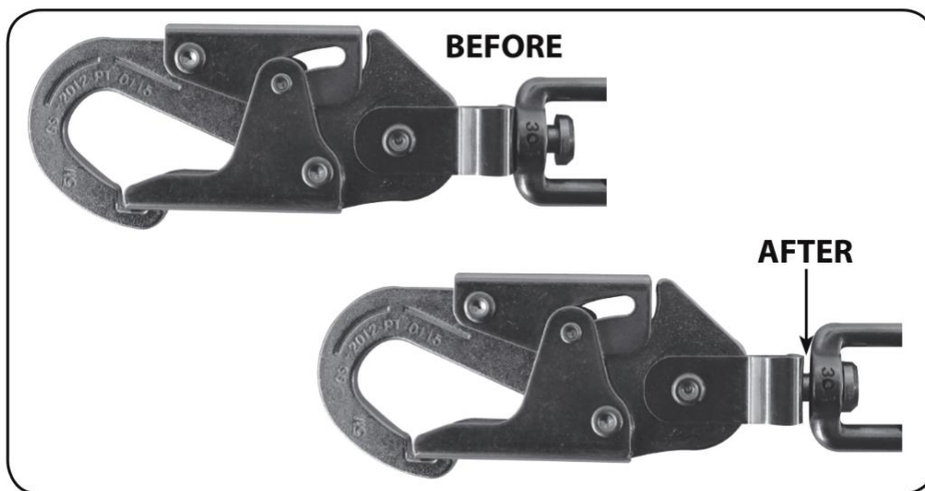
5.1 Before and After of Load Impact Indicator
