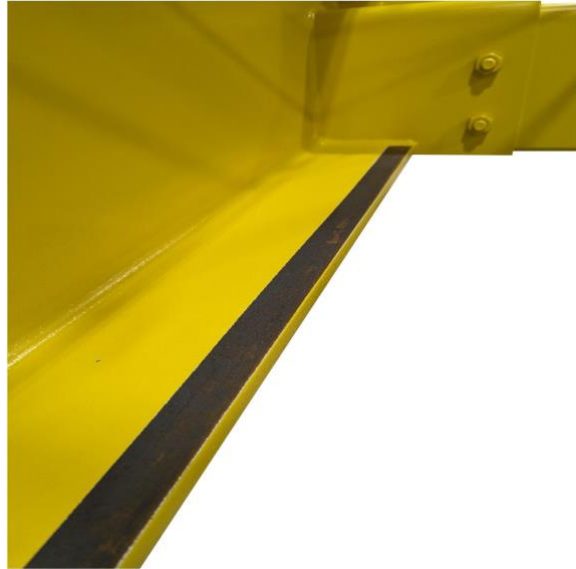
4.4.1 Taped Off Section on Crane
