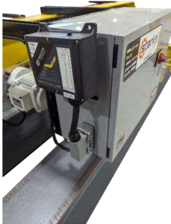
4.14.1 Radio Receiver Installed on Control Panel
